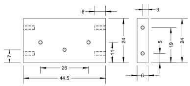
Frame spacers, 2 off, mild steel or brass drill all holes, 1.4mm and tap 10BA
