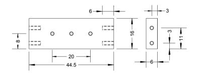
Frame spacers, 2 off, mild steel or brass drill all holes, 1.4mm and tap 10BA
