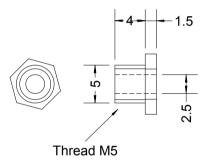
Piston rod and valve rods glands (4 off), Phosphor bronze, 6mm round or hex Scale twice full size
