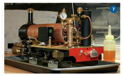
pipe was formed in aluminium and run from cab to smokebox.
