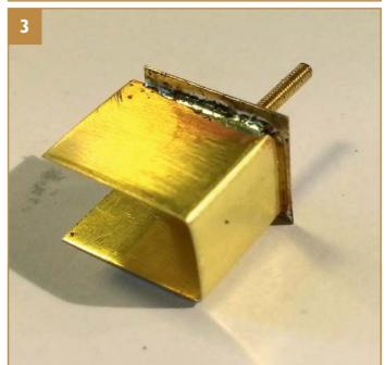
3. Solder the parts from steps one and two together to make the upper part of the lamp body. It's worth taking a little time to make sure that the sides are square. Don't worry if the lamp top is slightly off centre, you can use a file to trim the lip until it's all square.
