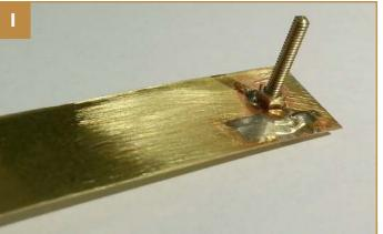
Take a strip of brass shim (approx 0.2mm thick and 11mm wide). Drill a hole to take a 10BA bolt dead centre and 6mm from the end. Solder the nut of the bolt into place and check that you haven't soldered the bolt solid. Screwing this bolt up and down will make the switch portion of circuit. Cut off the end of the strip with the bolt to a length of approx 14mm.
