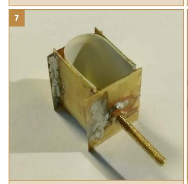
7. Cut a strip of very thin Plastikard and create a 'u' shape in the bottom of the lamp. Super glue this in place and drill the hole for the LED in the front of the lamp. This should be dead centre and just the right size so that the body of the LED fits through but not the collar at the base.
