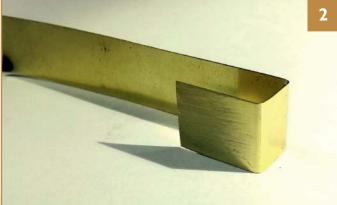
**2.** Take the strip and bend it into a 'n' shape with two 90 degree corners as shown in the photo. This will make the front and sides of the lamp, the folds should leave you with a front measuring 9mm wide, cut the sides to approximately 14mm length. These are oversize, but it's best to trim the lamp down when completed.
