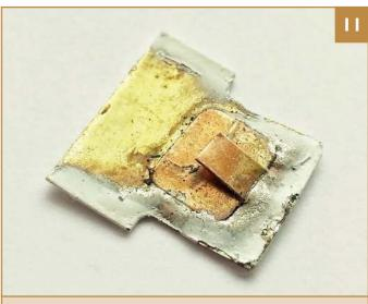
L. Cut the T shaped rear as per the picture and solder a small contact on the inside made from phosphor bronze
