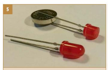
**5.** Prepare an LED by cutting the front off it. The working part of an LED is actually in the middle. If you hold it up to the light and look through it you can see the internal wires. Cut off the front just ahead of these wires. You don't have to do this, but it improves the look of the finished lamp.
