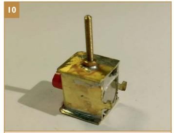
10. Now using a slitting disc in a mini drill trim the back of the lamp level with the rear of the batteries, leave two lugs, as per the picture, to secure the lamp rear.
