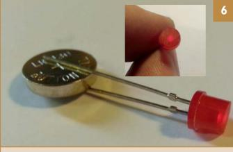
**6.** Having cut your LED you can polish up the front a little if you wish, and it's a good idea to put the leads across a watch battery just to check its still working. Connect the longer wire of the LED to the positive side of the battery, if all is well one battery should give dull glow from the LED.
