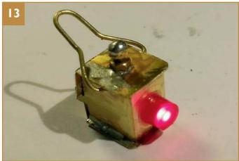
13. You can now assemble and test you lamp and decorate it as you see fit. I decided to trim the switch bolt and solder a nut to represent the vent on a oil lamp and add a handle. Finally paint and enjoy.
