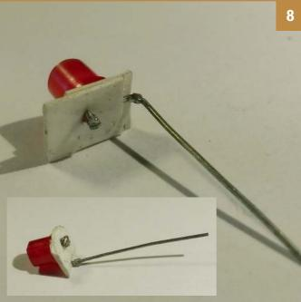
**8.** This next bit is fiddly. The longer LED lead needs bending to a right angle directly away from the shorter lead, this must be done as the lead emerges from the LED case.
