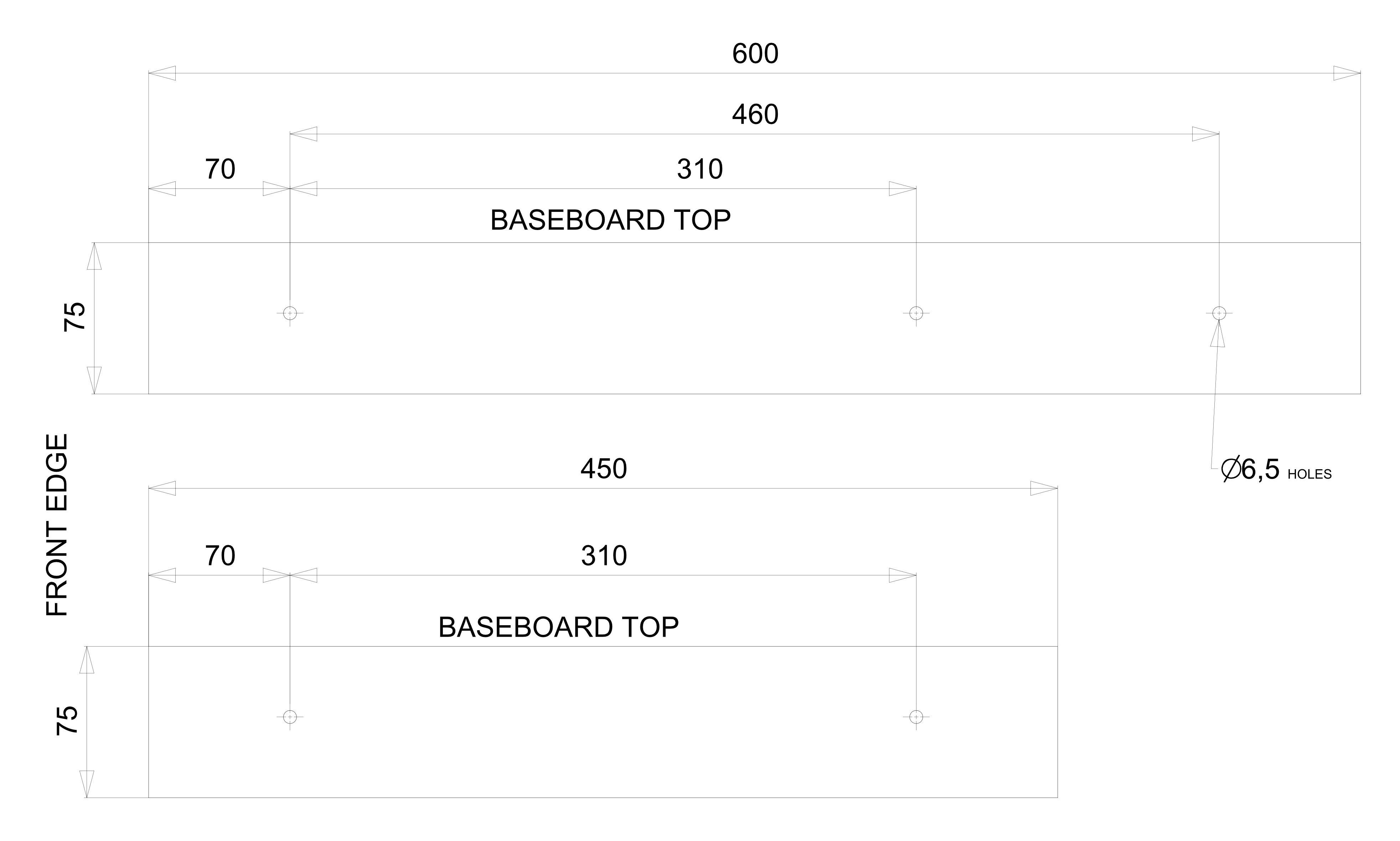
FOR OTHER BASEBOARDS WIDTHS. 750, 300 etc FOLLOW PATTERN. 40mm FROM TOP SURFACE, 70mm FROM FRONT AND BACK EDGE.
